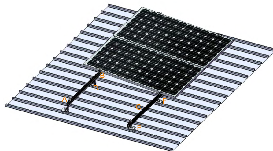
A. End Clamp B. Inter Clamp C. ECO/Elite Rail D. Rear leg E. Front leg F. Kliplok interface
