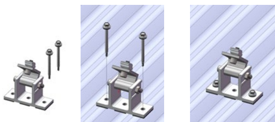
Figure 1 (Front Leg Installation with Two Screws)
