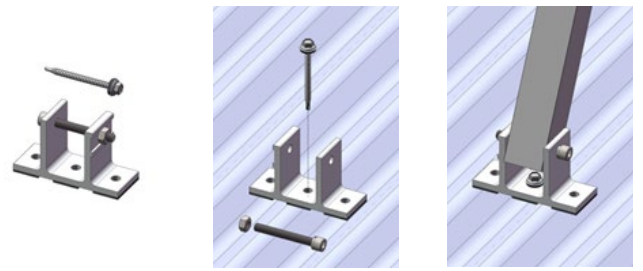
Figure 6 (Non-preassembly Rear Leg Installation with Single Screw)
