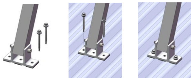
Figure 7 (Preassembly Rear Leg Installation with Two Screws)
