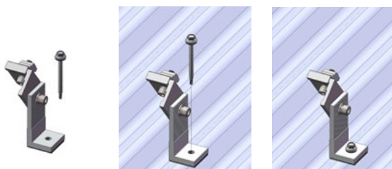
Figure 3 (Tin Foot Front Leg Installation)
