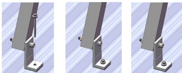
Figure 9 (Tin Foot Rear Leg Installation)
