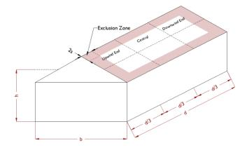
Exclusion zone for flush installation to be the minimum distance from the edge of the roof " $2 \times s$ ", where "s" is the gap between the underside of the panel and the roof. Refer to the exclusion zone (red area) on the above image.
