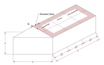
**Note 32.** Exclusion zone for flush installation to be the minimum distance from the edge of the roof "2 x s", where "s" is the gap between the underside of the panel and the roof.
