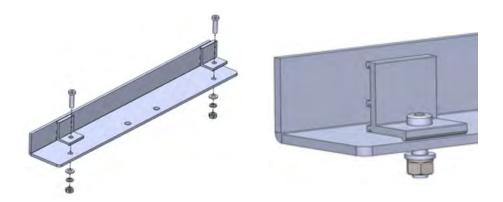
2) Connect the Angle Bracket to Rectangular Tube-Master with 8pcs U bolts, 16pcs M10 nuts, 16pcs spring washer, 16pcs washer as shown in the figure below.
