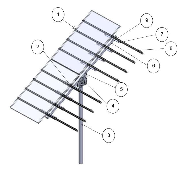
1. End Clamp2. Inter Clamp3. PM4-A Pole4. Steel Cap Assembly5. Adjustable Tube6. Rectangular Tube-Master7. Angle Bracket8. ECO-Rail9. U bolt for Tube110
