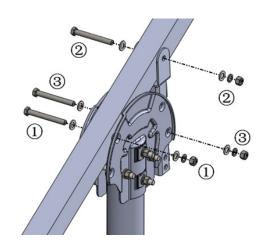
Fasten the Steel Cap Assembly to Pipe with M20\*210, M20\*160 Hex Bolt, keep the Rectangular Tube-Master parallel to the south-north by adjust the Steel Cap Assembly.
