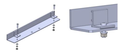
Connect the Angle Bracket to Rectangular Tube-Master with 6 pcs U bolts, 12 pcs M10 nuts, 12 pcs spring washer 10, 12 pcs plain washer 10 as shown in the figure below.
