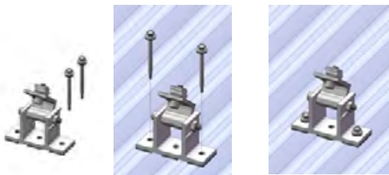
Figure 1 (Front Leg Installation with Two Screws)
