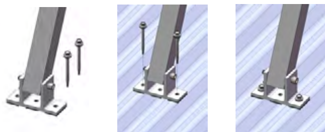
Figure 7 (Preassembly Rear Leg Installation with Two Screws)
