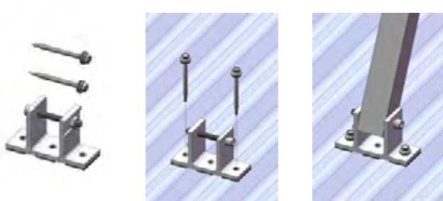
Figure 5 (Non-preassembly Rear Leg Installation with Two Screws)
