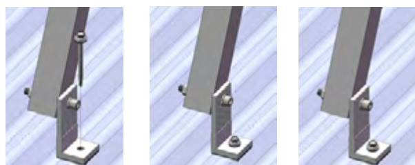
Figure 9 (Tin Foot Rear Leg Installation)
