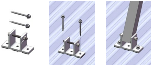
Figure 5 (Non-preassembly Rear Leg Installation with Two Screws)
