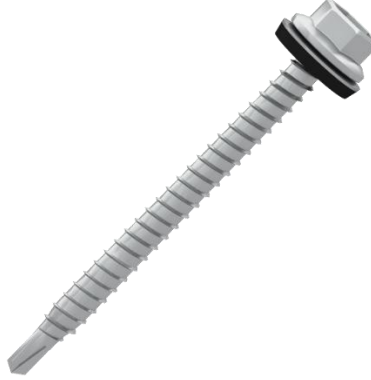
Self-drilling Universal Screw, Buildex 14-11 x 70 Hex Head Zips Climaseal 5 with 16 mm ABW Part No.: US-6.3/70/C5-BW/BX (bar code: 13-14011-064)
