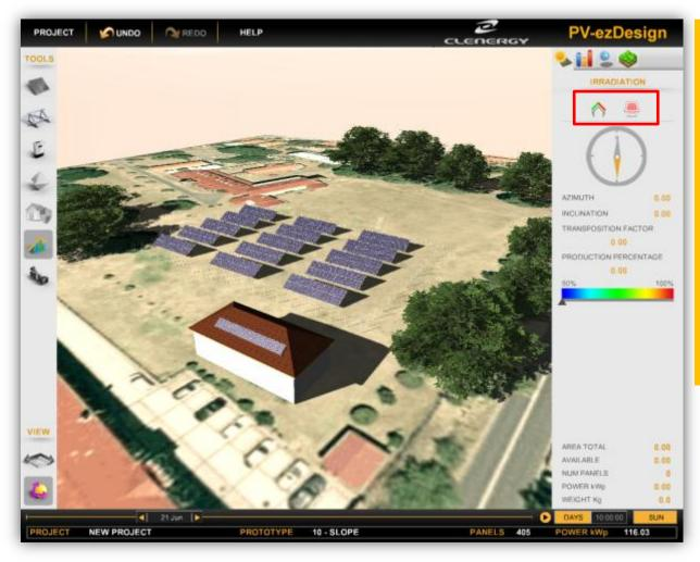
: Slope selection. It used for a face of a pitch roof and the irradiation data for the selected roof will be given by clicking on this icon.
