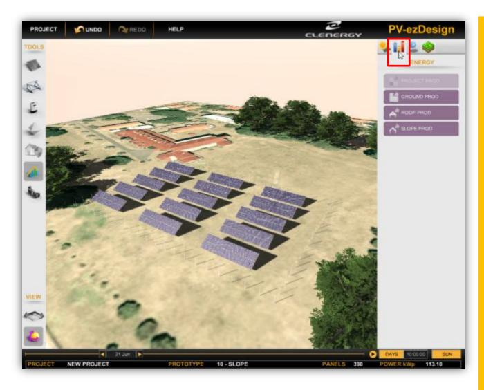
A report illustrating a comparison between the designed system and optimal condition in terms of global irradiation and electricity production can be given by clicking on "PVGIS ENERGY".
