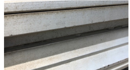
Figure 3: 6005CL alloy – After 21 years
