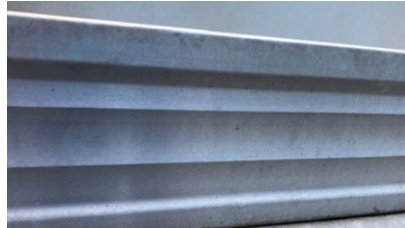
Figure 2: 6005CL alloy – After 6 years
